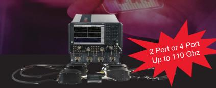
The better alternative is a preconfigured solution that includes a two- or four-port network analyzer along with the necessary millimeter-wave cabling, frequency extenders, and test-set controller.
